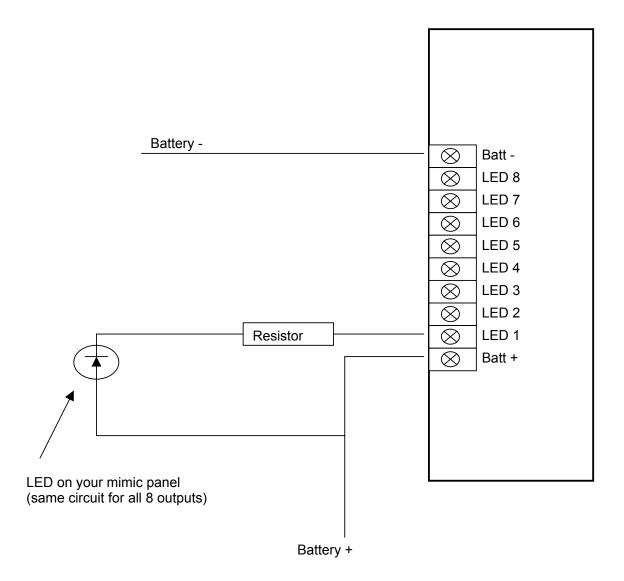
The led output circuit is repeated for all outputs.
