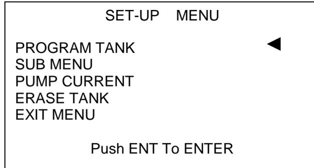
Scroll to PROGRAM TANK and press the ENT key.
