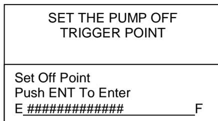
Use the Select Up or Down key to move the Pump Off point to the desired level. Press the ENT key to set this as the Pump OFF point.
