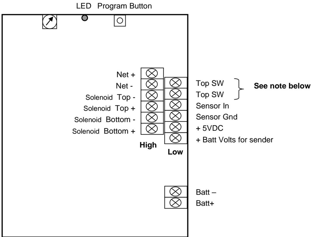
**NOTE:** If the tank emergency top switch is not fitted then a link must be placed between the two "Top Switch" terminals
