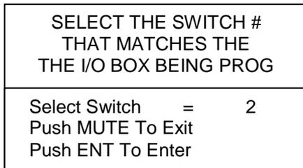
Use the Select Up or Down key to change the Switch number which corresponds to the I/O unit you wish to program (refer to Table 1 on page 12) for Switch number. Once the Switch number has been selected press the ENT key.
