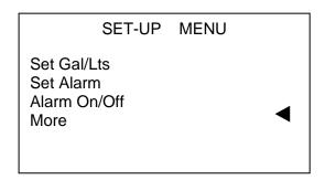
Use the Scroll button to Scroll to the function and push the Enter button.
