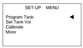
Push the Enter/Pump button to select the tank Name or scroll to another function.
