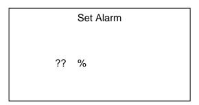
The alarm point is a percentage of the tank e.g. If the tank Volume is set to 100 lts and the alarm set to 10% then the alarm will sound at 10 lts
