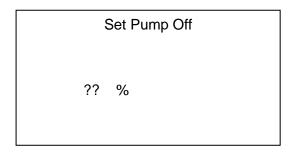
The pump Off point is a percentage of the tank e.g. If the tank Volume is set to 100 lts and the pump off point is set to 10% then the pump will turn off when the tank reaches 10 lts
