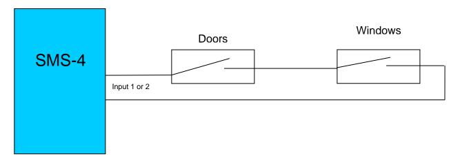
Send command text: Change input? to Door Sensor Send command text: Make Door Sensor latching Send command text: Make Door Sensor active open (sensors are normally closed and go open when activated)
